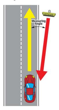
Figure 6-3. Radar Speed Errors
