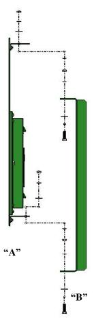
Figure 6-2. Connecting DFB Sign to Bracket
