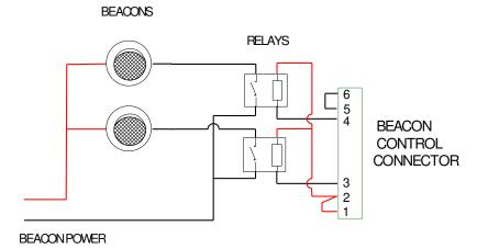
RECOMMENDED WIRING 25W OR MORE, OR AC POWER DISPLAY BEACON TIMING
