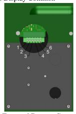
Figure 6-5. External Beacon Connections
