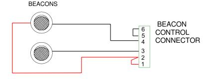
RECOMMENDED WIRING BEACONS 12W or LESS, 12VDC DISPLAY BEACON TIMING
