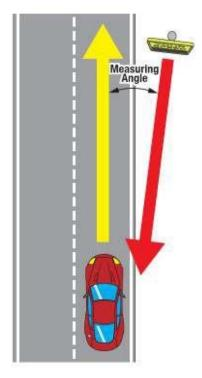
Figure 6-2. Radar Speed Errors
